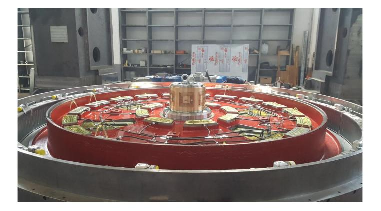
A hydrostatic rotary table is a specialized type of rotary table that is designed specially to achieve high precision and stiffness by utilizing a hydrostatic bearing system.
